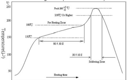
Remark: The peak temperature of soldering heat is 260 +5/-0 °C for 10 seconds
